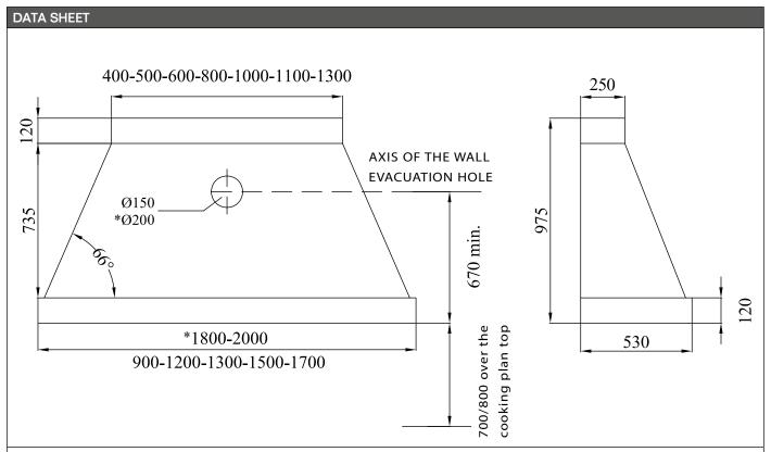
Please do not connect the hood to an air extraction pipe smaller than the advised one. Danger of a general bad working of the appliance and overheating of the engine. In the case the extraction pipe cannot be  $\emptyset$  200mm (1200mc/h) and the hood is larger than 180 cm, we suggest to order the hood with an engine apt to air extraction pipe  $\emptyset$  150mm (900mc/h)
